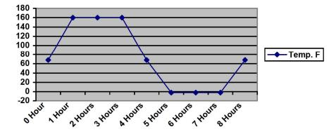
The above chart is representative of the average exterior temperature of the test specimen during the three (3) thermal performance cycles.
